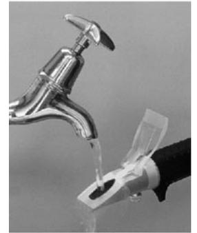
The prism surface could be damaged by strong alkalis or acids if left in contact for long periods of time. Clean samples from the prism as soon as practicable.
